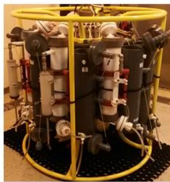
Figure 4: a) Online Photometric Ultraviolet Spectrophotometer (OPUS) build by TriOS GmbH (Oldenburg); b) OPUS was mounted at the bottom of the Rosette water sampler; c) Rosette water sampler equipped with the Automatic Flow Injection System (AFIS); d) mini DOTs were mounted inside the AFIS bottles.
